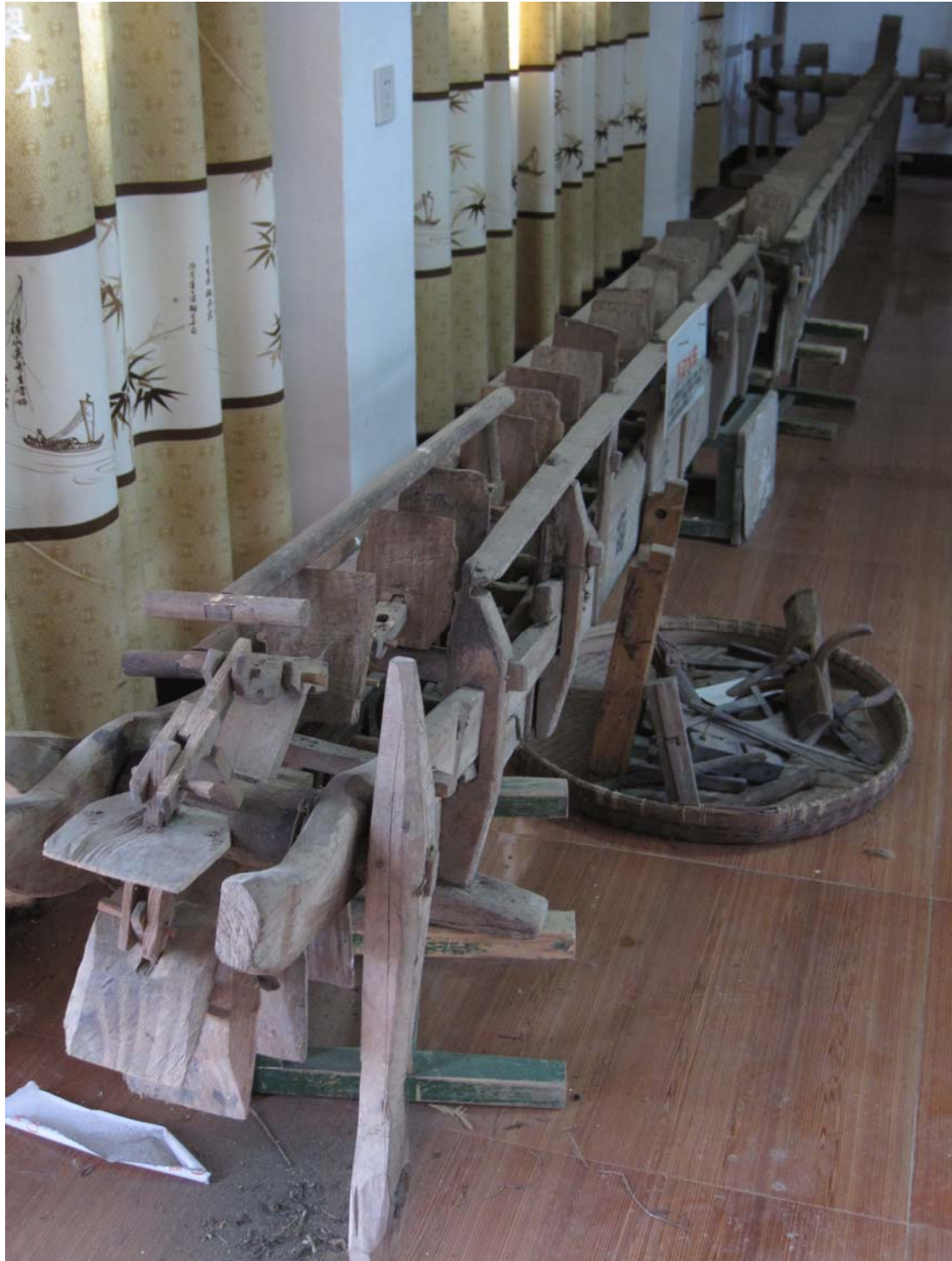
Figure 4 Foot-driven Dragon-Bone Water Lift, photographed in Zhaitan Museum on 26 September 2010
