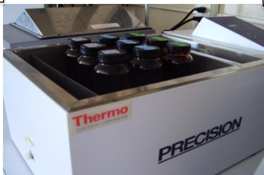
Water bath at 55°C with Amber bottles containing pretreated biomass and enzyme mixture
