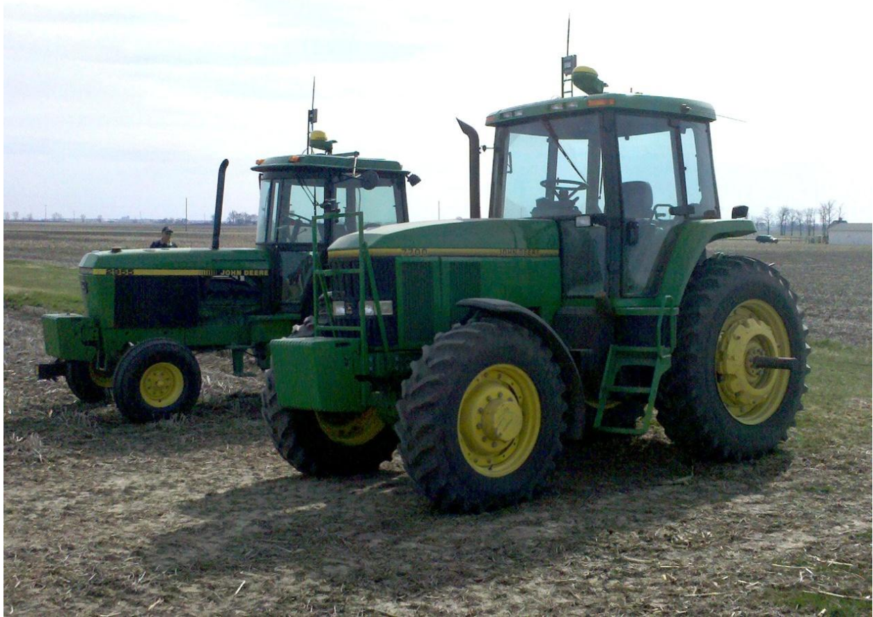
Figure 12. Two tractors fitted with GPS hardware and radios for field tests.
