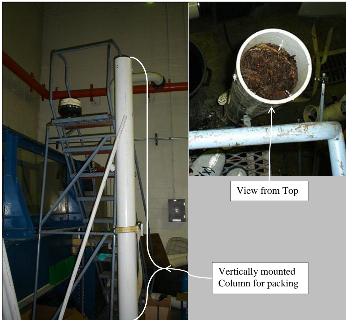
Figure 5.8. Column mounted vertically during packing procedure.
