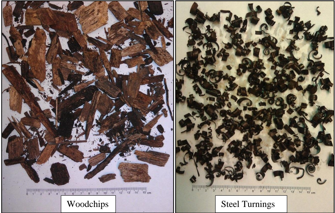
Figure 5.9. Size distribution of Steel Shavings and Woodchips.
