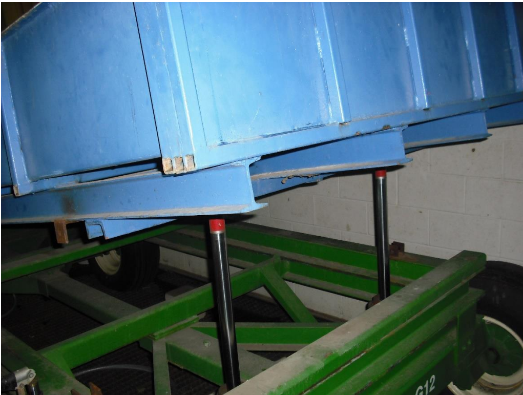
Figure 4.2: Hydraulic cylinders elevating soil bed to 15% slope.
