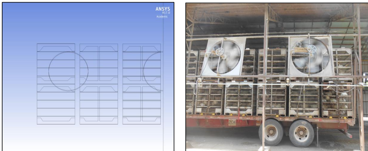
Figure 2.1: Comparison of model geometry and trailer at the test site. Vertical plane to the right in model geometry has symmetry boundary condition
