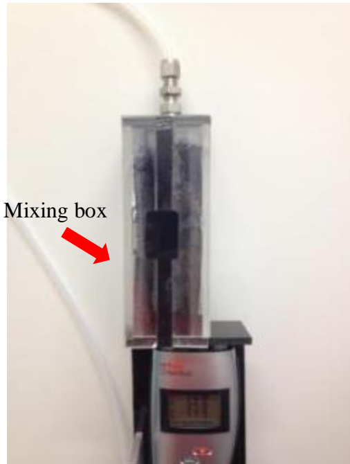
Figure C.2: Mixing box with electronic temperature and relative humidity sensor attached. results. The general equipment required to perform the calibration is shown in Figure C.3.
