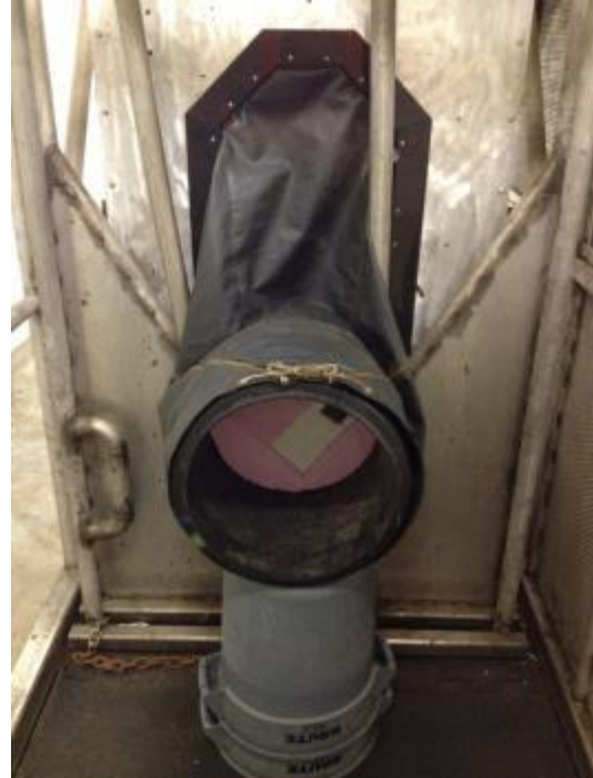
Figure 3.7: Styrofoam board within a section of 14" diameter plastic tube acts as an animal's head and sufficiently seals the hood.
