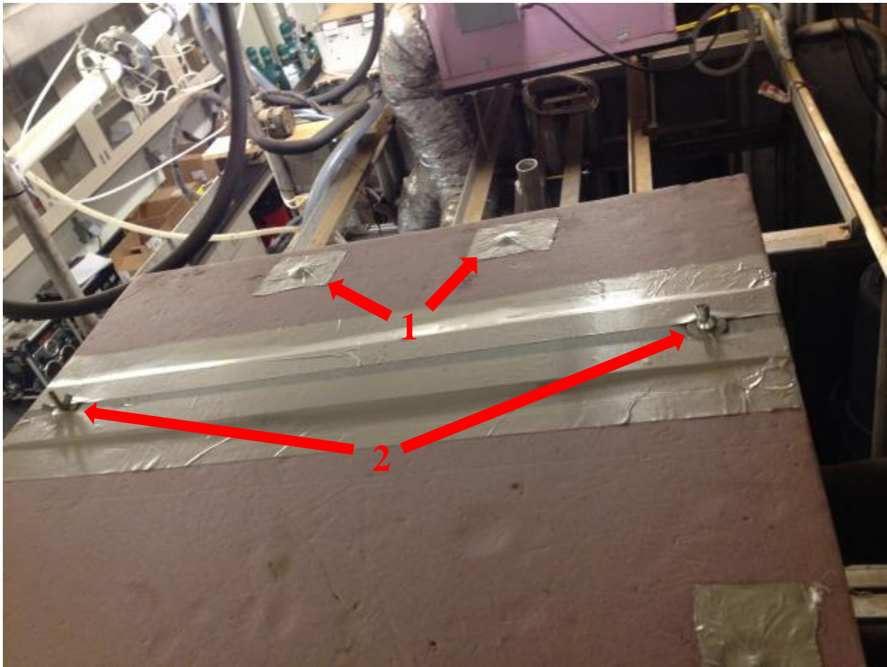
Figure 4.5: Top view of CACU with filter cover, sealed with tape. Please note location of screws for cover taped over (1) and butterfly nuts (2).
