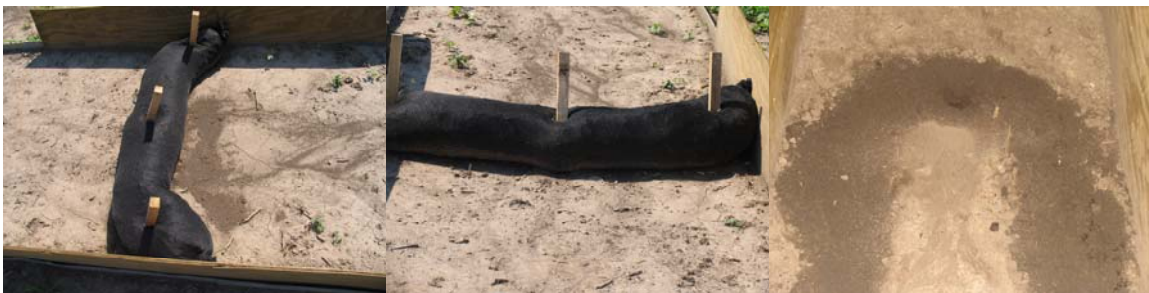
Figure 5.12. Compost sock in use and the resulting deposition pattern that could affect flow.
