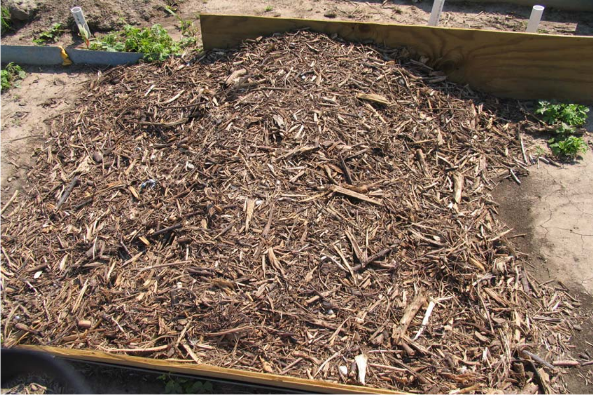
Figure 4.3. Compost filter berm at field study site.
