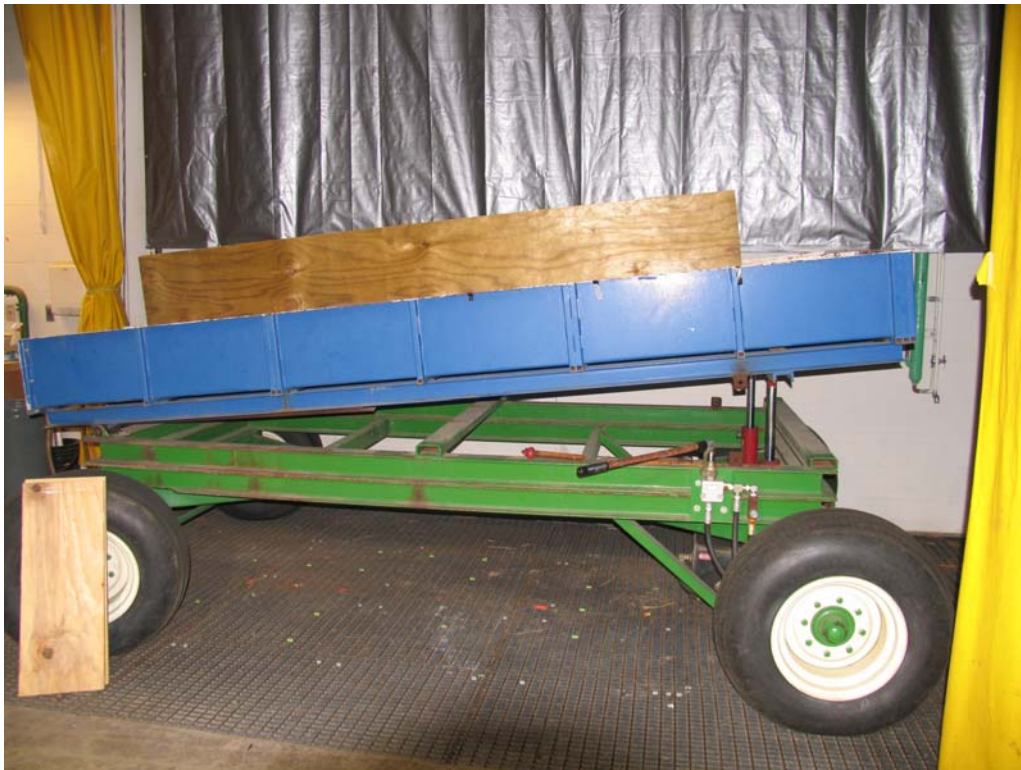
Figure 4.12. Tilting bed soil wagons used under rainfall simulator.
