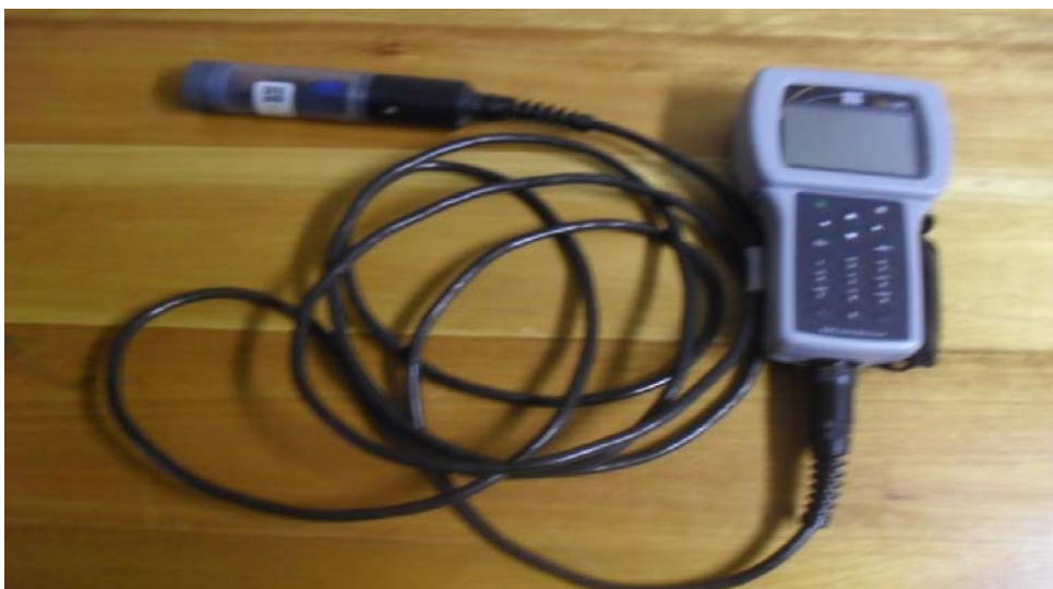
Figure 3.7: YSI meter (MPS 556) used for measuring some of the water quality parameters.
