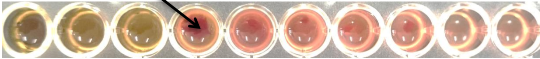
Figure (3.1): Minimum inhibitory concentration determination using microbroth dilution method with TTC as indicator.
