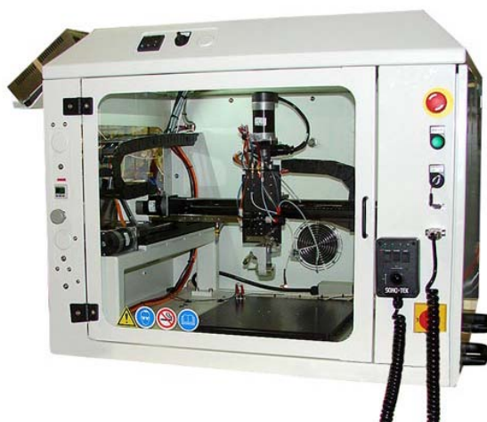
Figure A.3 Sonotek Exacta-Coat sprayer controlled by X-Y-Z Robot.
