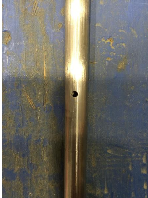
Figure 3.4 Defect on a mock failed fuel rod.
