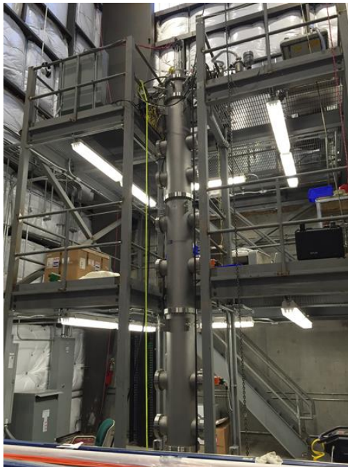
Figure 3.3 An example of a sealed chamber to accommodate the mock fuel rod assembly.
