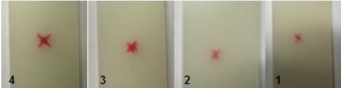
Figure 3.3. Damage area in Glass fiber specimens subject to low velocity impact damage
