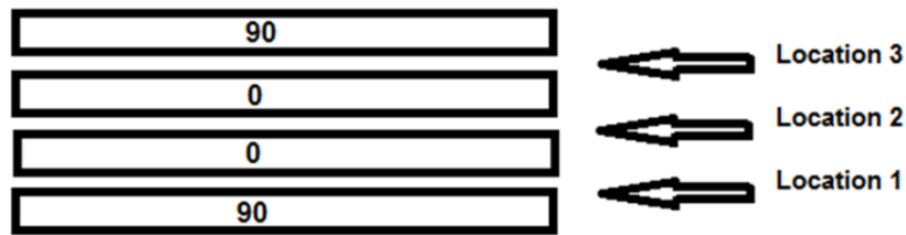
Figure 4.2. Specimen layup and planned delamination locations.
