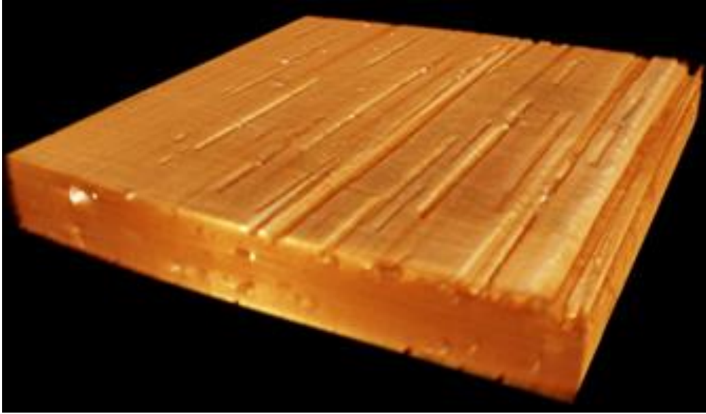
Figure 4.12. 1X 3D X-ray Image of cross-ply specimen subject to a 15000N Tensile Force
