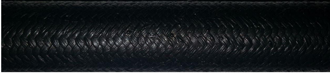
Figure 3.7 Roughness structure on the SiC Fuel Rod
