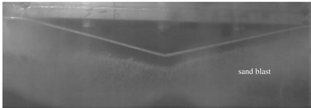
Figure 3.11 Side view of ejected sand interacting with V-shaped hull during blast event.
