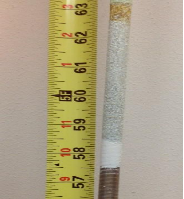
Figure 6.9: Nano-particle depositions on rough and smooth section of 0.5% Nanofluid
