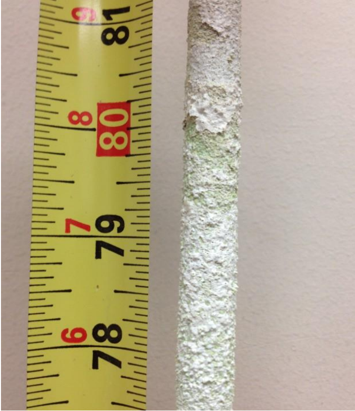
Figure 6.8: Nano-particle depositions on smooth section of 3-D roughness
