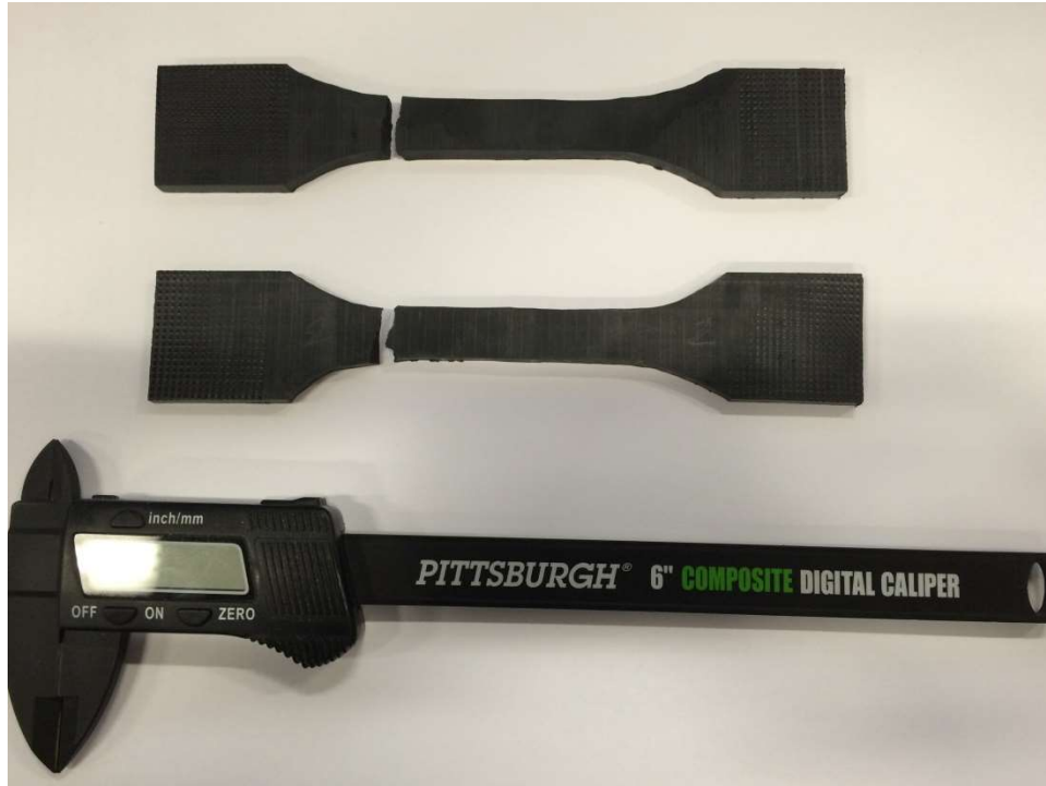
Figure 5.8: Tensile test specimen after fracture
