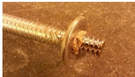
Figure 3.5: FSW tool with one washer as a shoulder
