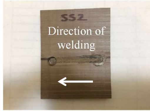
Figure 4.19: Specimen made using stationary shoulder
