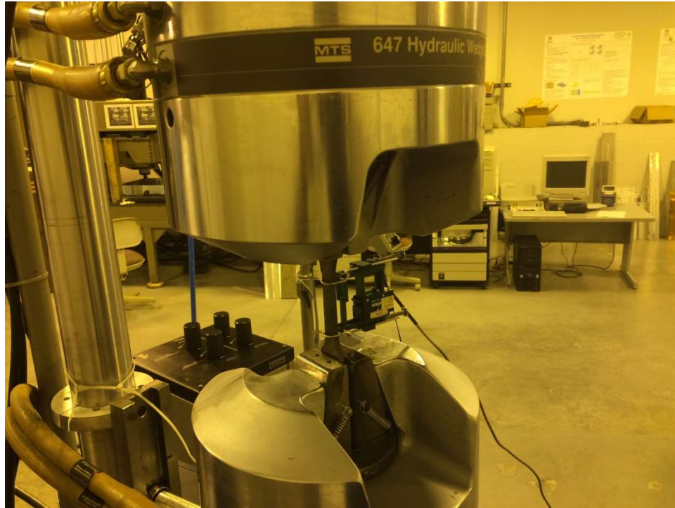
Figure 5.7: Tensile test arrangement of PEEK samples using MTS
