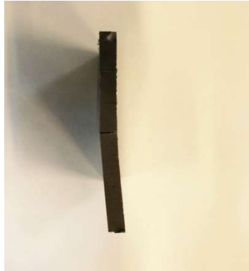
Figure 4.9: Welded PPS sample with uneven expansion.
