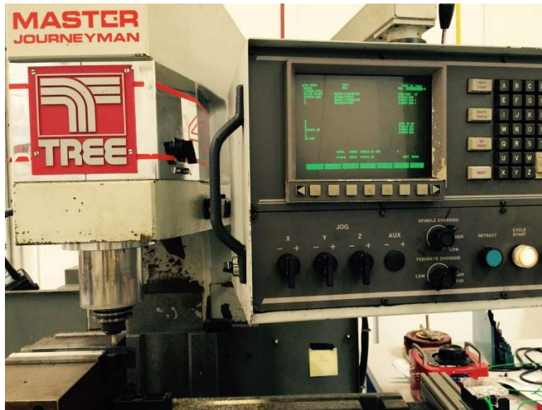
Figure 3.3: Journeyman 425 Milling machine with Dynapath CNC control
