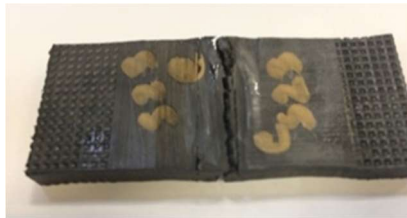
Figure 5.9: Failure of welded sample at the weld interphase.
