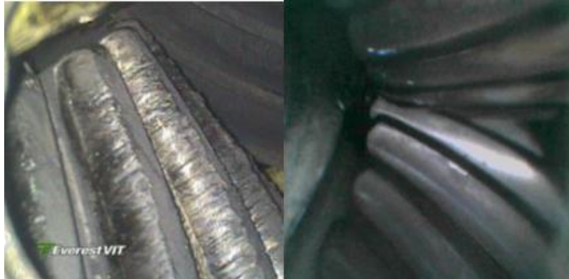
Figure 4.1 A comparison, from a previous experiment, of worn gear teeth (left) to healthy teeth (right)
