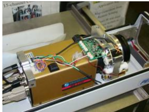
Figure 3.3. Camera, compass and lens controller inside the camera housing.
