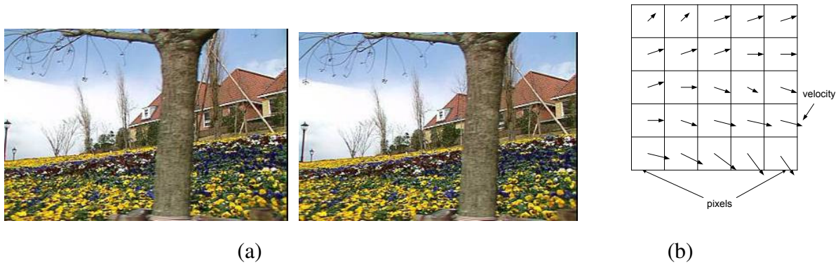
Figure 4.10. (a) A pair of adjacent images, (b) computed velocities of every pixel.
