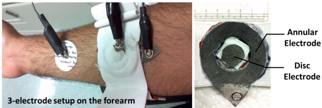
Figure 23: (a) 3-electrode setup on the fore arm with concentric ring electrode (CRE) pair and Ag-AgCl counter electrode, (b) CRE made with flock electrode
