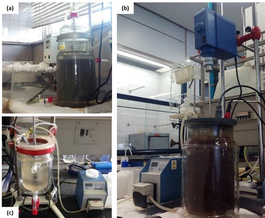
Figure 5.1. Photos of the three reactors used in this study: (a) continuous fermentation reactor, (b) sequencing-batch biomass selection reactor, and (c) fed-batch PHA accumulation reactor.
