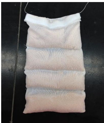
Figure 4.2. One of three mesh bags that were deployed into the continuous AnMBR system containing approximately 400 g of Purolite® TANEX™ each for a total dosage of 100 g/L.
