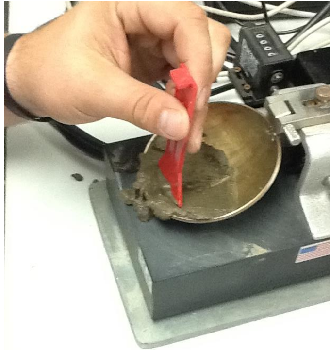
Figure 4.7: Grooving of a liquid limit sample
