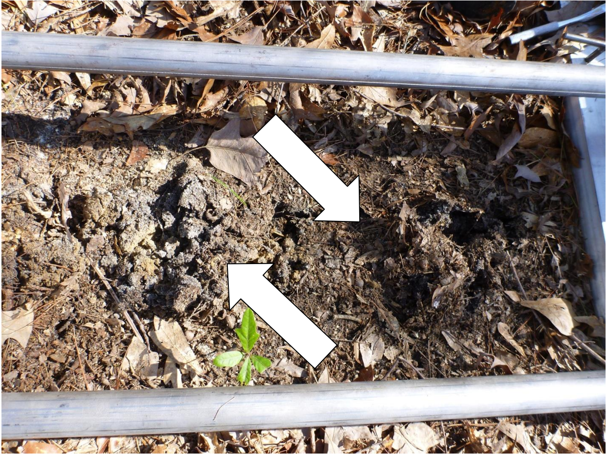
Figure 4.3: Soil displacement after two VASST tests (tests indicated by arrows)
