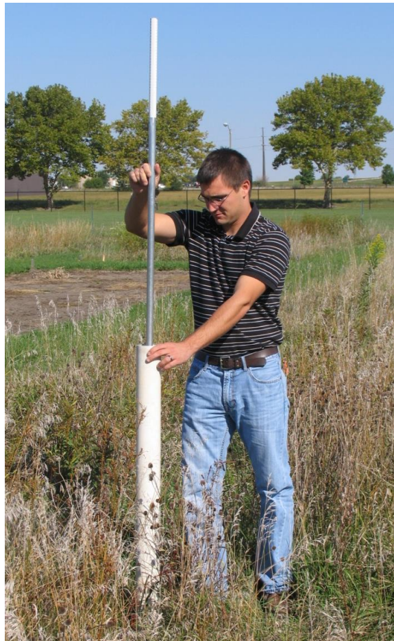
Figure 4.5: Example of drop-cone test
