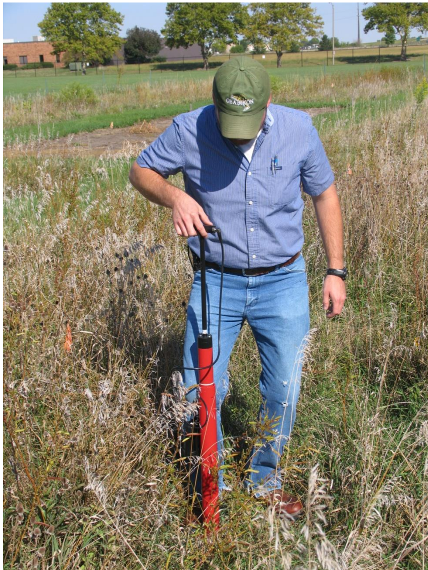
Figure 4.6: Example of Clegg impact test
