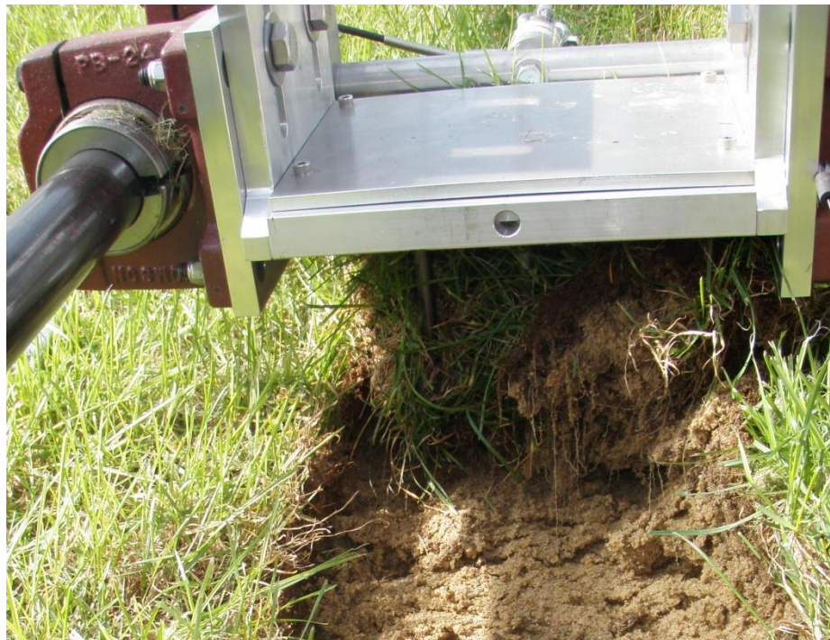
Figure 3.2: Tire analog during VASST test
