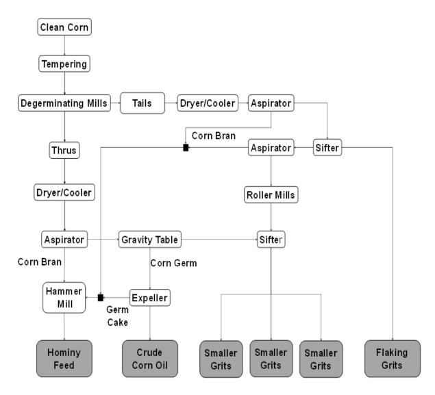
Fig. D.2. Dry milling process flow.
