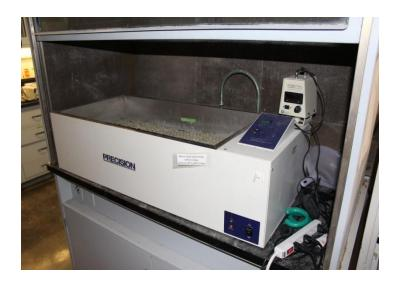
Water bath for liquefaction and fermentation
