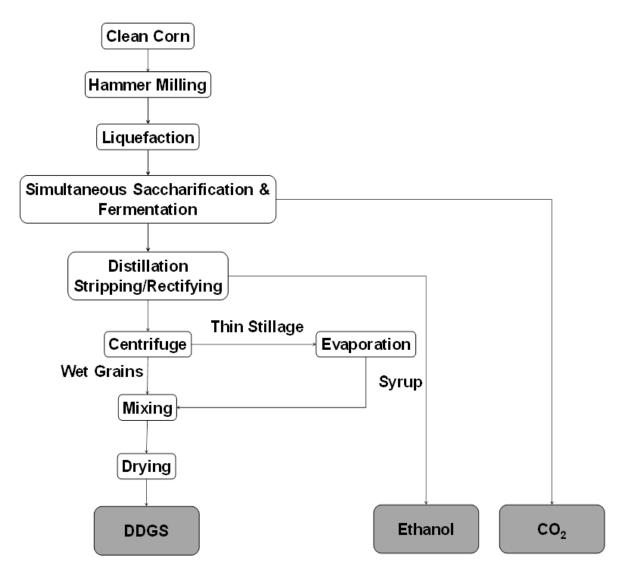
Fig. D.3. Dry grind process flow.
