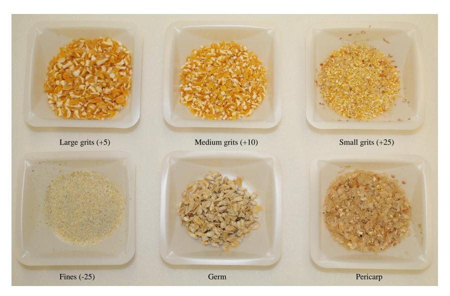
Fig. 6.2. Various coproducts from 100 g dry milling of Hard1 corn.
