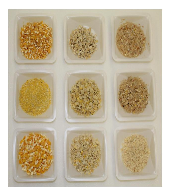
**Fig. 6.3.** Comparison of large grits, germ and pericarp (left to right) from 100 g dry milling protocol (top), 1 kg protocol (middle) and commercial samples (bottom).
