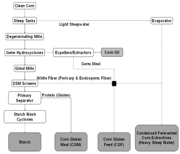
Fig. D.1. Wet milling process flow.
