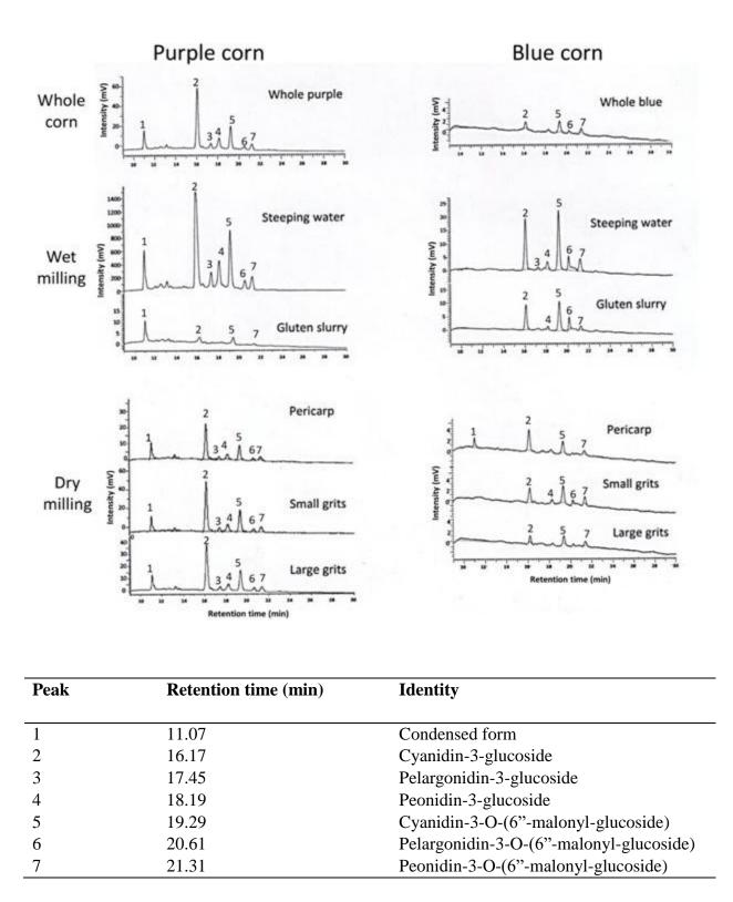
**Fig. 4.1.** HPLC chromatograms of acidified water extracts from purple and blue corn dry milling, wet milling fractions and whole corn at 520 nm and possible identities of main peaks by LC/MS.
