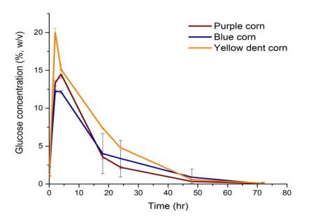
**Fig. 3.2.** Respective glucose concentrations during fermentation. Error bars are  $\pm 1$  standard deviation.
