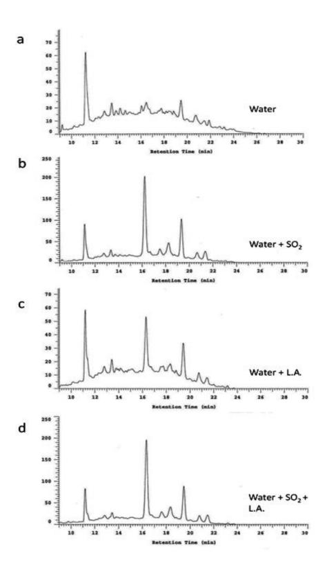
**Fig. 5.3.** HPLC chromatograms of corn pericarp steeping combinations with only water (a) water plus SO<sub>2</sub> (b) water plus L.A. (c) and water plus SO<sub>2</sub> and L.A. (d) at 280 nm.
