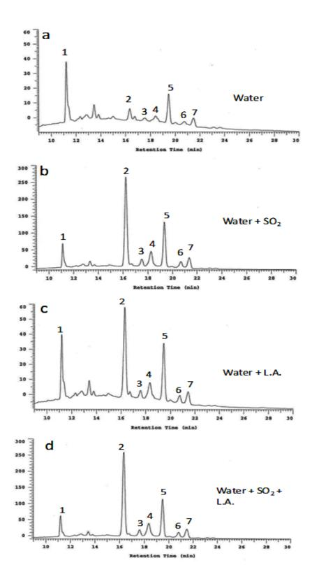
**Fig. 5.7.** HPLC chromatographs for all treatments at 520 nm. The peaks indicate the following: 1: Condensed form; 2: C3G; 3: P3G; 4: Peo3G; 5: C36MG; 6: P36OMG and 7: Peo36OMG.
