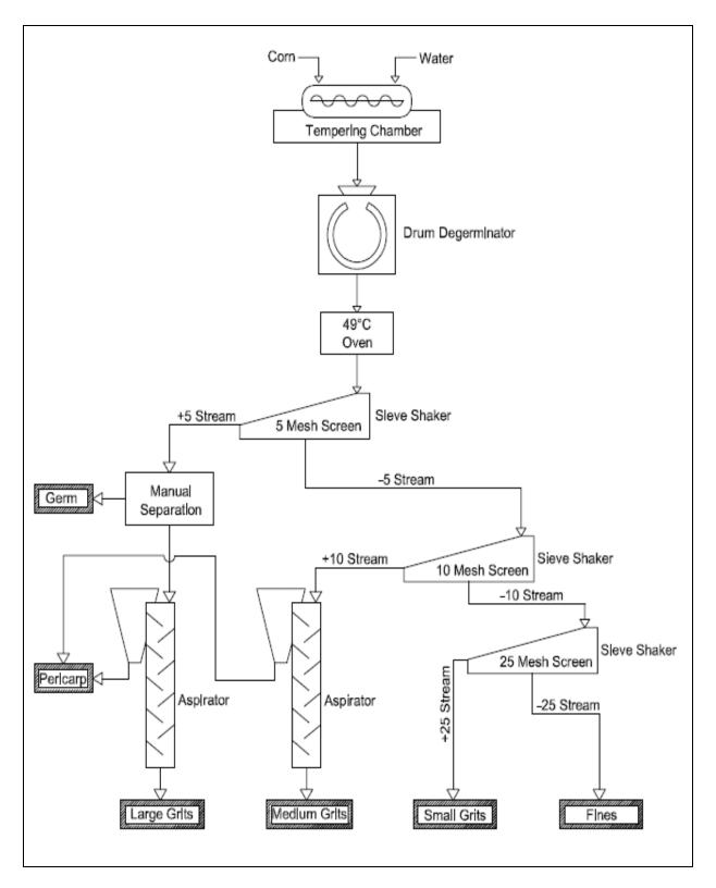
Fig. 6.1. Process flow in the 100 g dry milling protocol.
