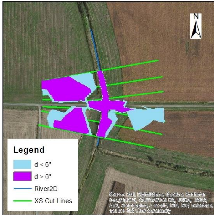
Figure 5.14: Flood inundation map for 25-year flood in Franklin LWC.
