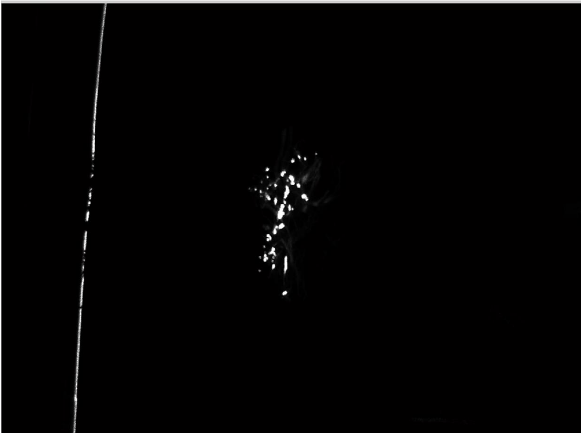
Figure 19: The original system used a laser sheet that was slanted downward at a 45 degree angle, causing the line on the left as shown in this figure. This problem was eliminated by adjusting the laser sheet to a horizontal attitude.
