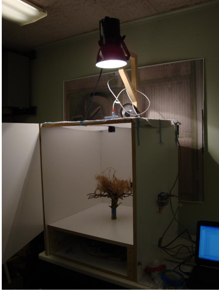
Figure 25: Photo of the current corn root imaging box (CRIB) that features diffuse lighting and an automated system that rotates the roots.
