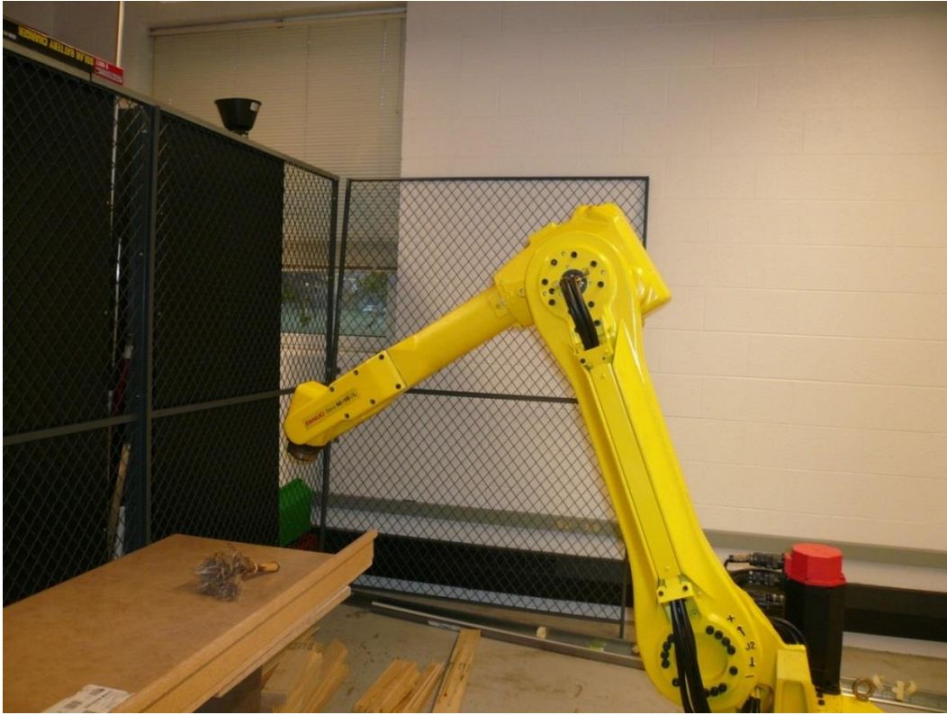
Figure 6: FANUC M-16iL industrial robotic arm. This robot was initially targeted for handling of corn roots and ears, but this method was replaced by a Corn Root Imaging Box that simplifies using structure lighting and image acquisition.
