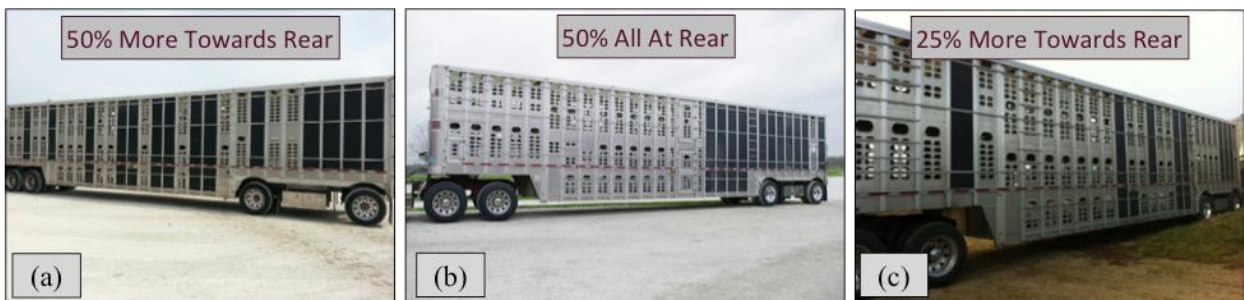
Figure 3-13. Alternative boarding placement arrangements assessed in cooperation with outside temperature and monitoring completion, for temperature -7 to 9°C (20 to 49°F). (a) 50% boarding more towards rear, (b) 50% boarding all at rear, and (c) 25% boarding more towards rear. Left indicates the front of the trailer and right indicates the back of the trailer.
