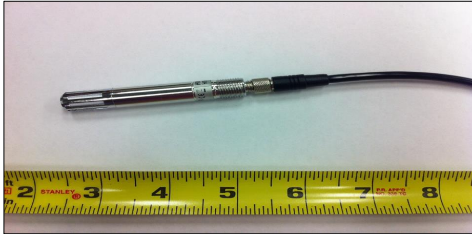
Figure 3-7. Zone-centered air temperature and relative humidity (RH) sensor (Vaisala HMP60, Vaisala). 6 zone-centered air temperature and RH sensors were implemented at the central area at ceiling within each 6 cross-sections to measure the central air temperature and relative humidity of each trailer zone.
