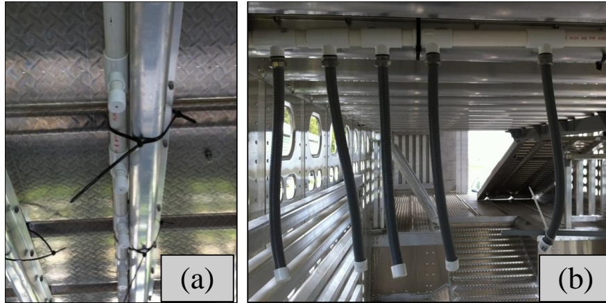
Figure 3-3. Mounted PVC pipes for thermistors in trailer. (a) Mounted PVC on ceiling in front and rear zones, and (b) the PVC pipes fixed on the ceiling with 14 flex conduits hanging down. The vertical placement with respect to the height above the pigs' back was consistent for all zones within the trailer.
