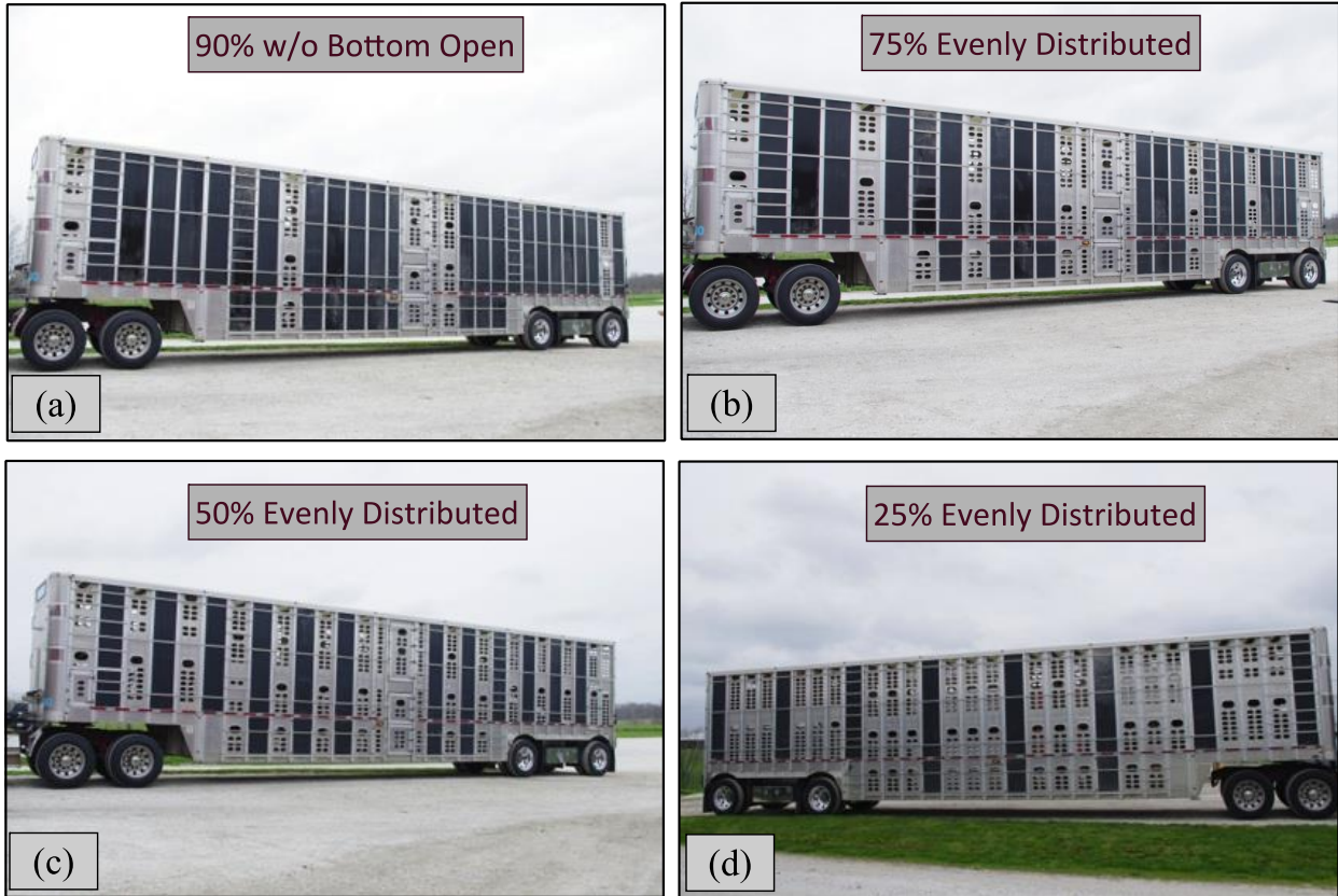
Figure 3-12. TQA typical boarding percentage arrangements assessed for cold weather conditions. (a) 90% boarding with bottom covered, (b) 75% boarding coverage evenly distributed, (c) 50% boarding coverage evenly distributed, and (d) 25% boarding coverage evenly distributed.
