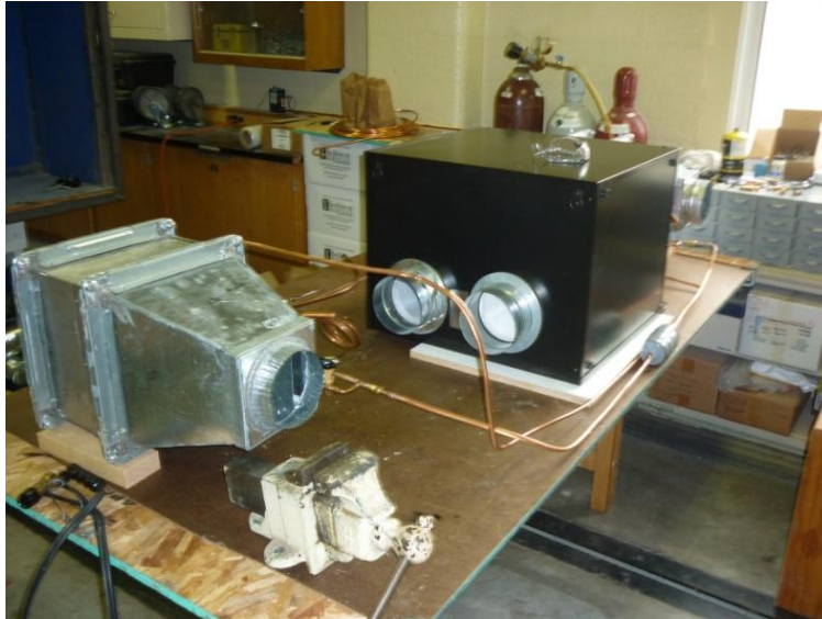
Figure 2-15. View of ERV, supply ductwork, and filter dryer.
