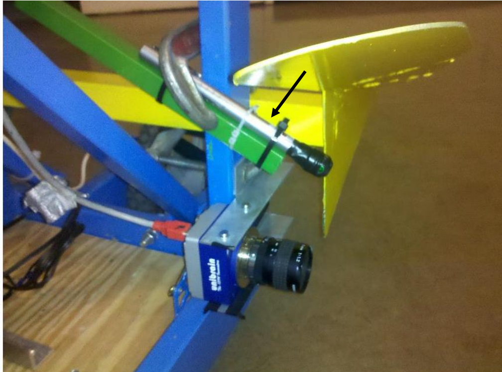
Figure 14: Imaging system mounted on a cart. Note the slanted laser sheet generator above the camera.
