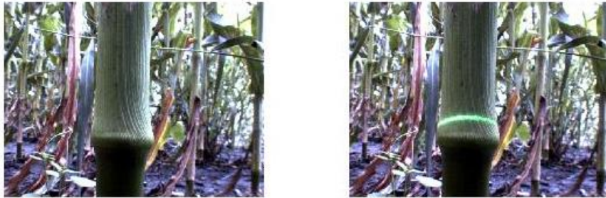
Figure 19: Image subtraction approach of the ILS in a real field environment
