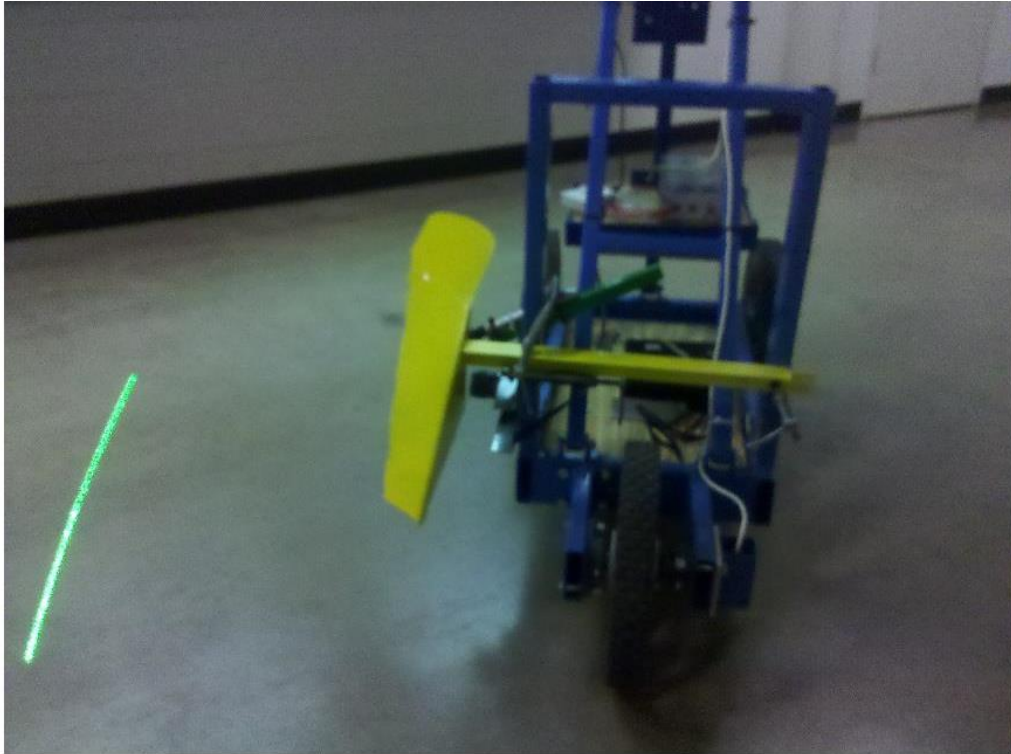
Figure 15: Measurement cart showing the deflection blade and projected laser sheet
