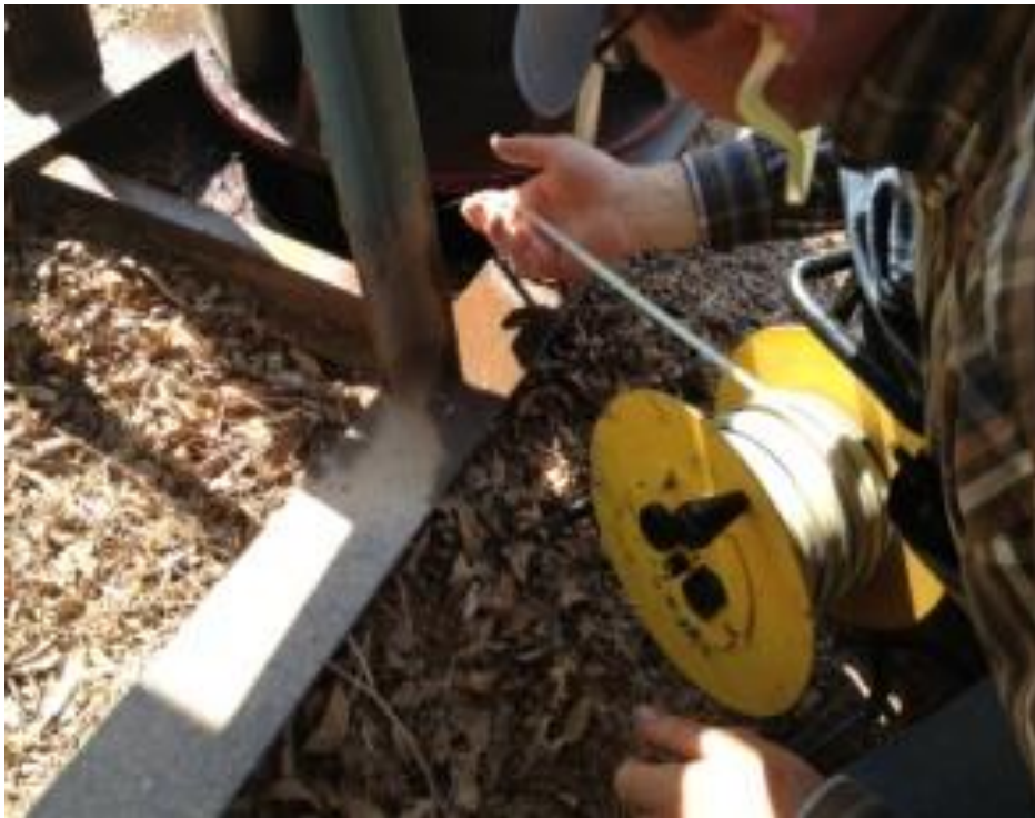
Figure 12. Measuring PWL of a Well Pumping Plant Using a Sounding Tape.
