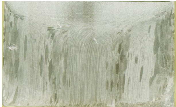
Figure 5.2 A cross section of the remnant aluminum alloy sample after etching.
