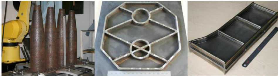
Figure 1.3 Parts produced by the wire and arc additive manufacturing process [5].
