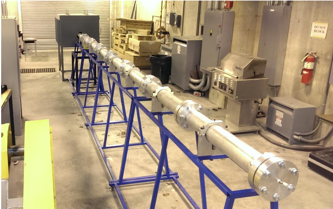
Figure 2.4 Fully-assembled shock tube and supporting frame with roller bearings.
