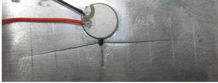
Figure 6.35: PWAS bonded next to a 20 mm long fatigue crack
