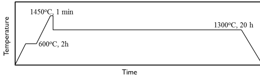
Figure 3.10 Two-step sintering profile for BZCYYb ceramic.
