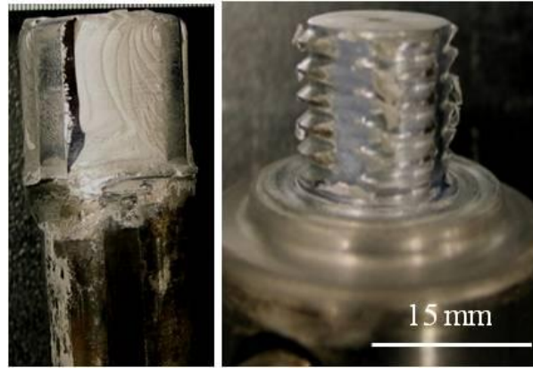
Figure 4.12 Unthreaded pin (left) and threaded pin (right) showing material adhering to flats (or not)
