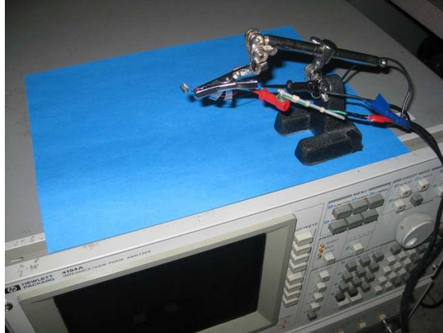
Figure 291: 300 kHz FBG ring sensor - setup configuration
