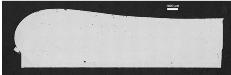
Figure 8. Representative René 80 deposit produced by SLE.
