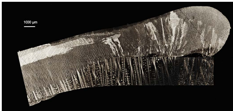
Figure 11. Warping of SLE deposit due to higher scanning speed.
