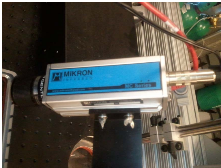
Figure 51. Mikron IR camera mounted on top of glovebox.
