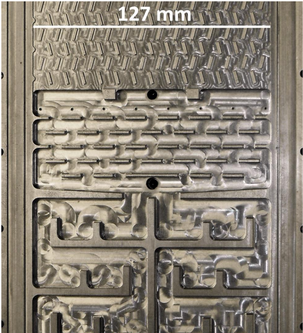
Figure 3.9 : Branched tray solution plate features in rectifier (top), analyzer (middle), and desorber (bottom)
