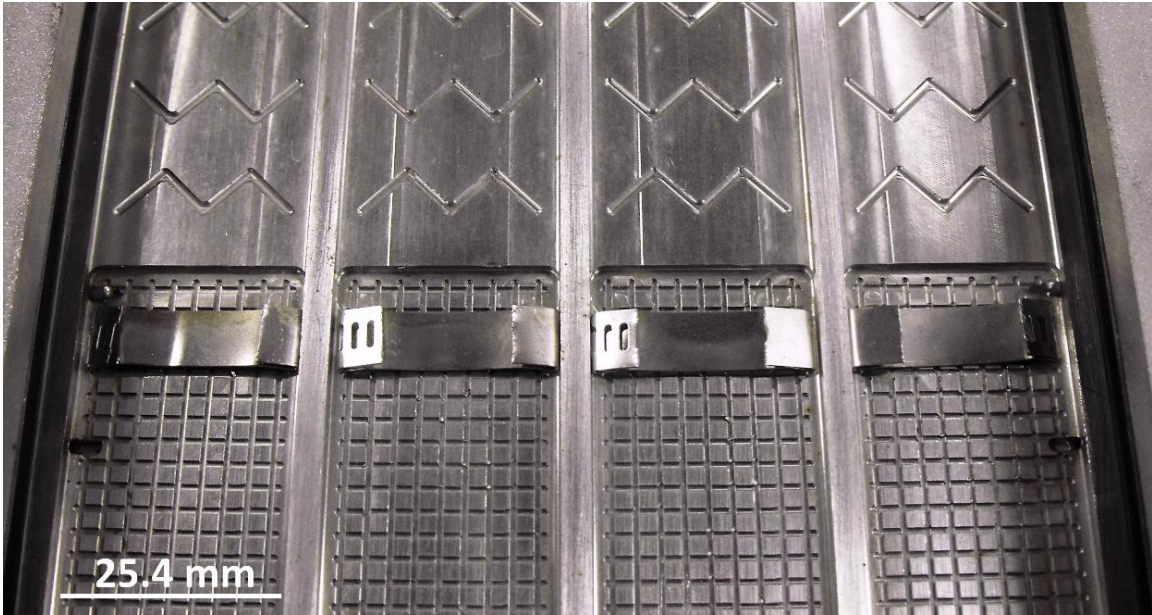
Figure 3.8 : Vertical column surface treatment in rectifier (top) and desorber-analyzer (bottom); solution distributors also shown
