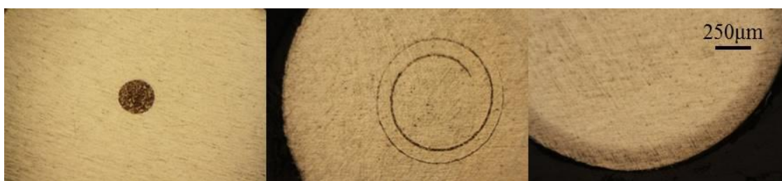
Figure 3.21 Bottom cross-section of flat die extruded wire (left) Center marker, (middle) 1/3 radius marker, (right) 2/3 radius marker
