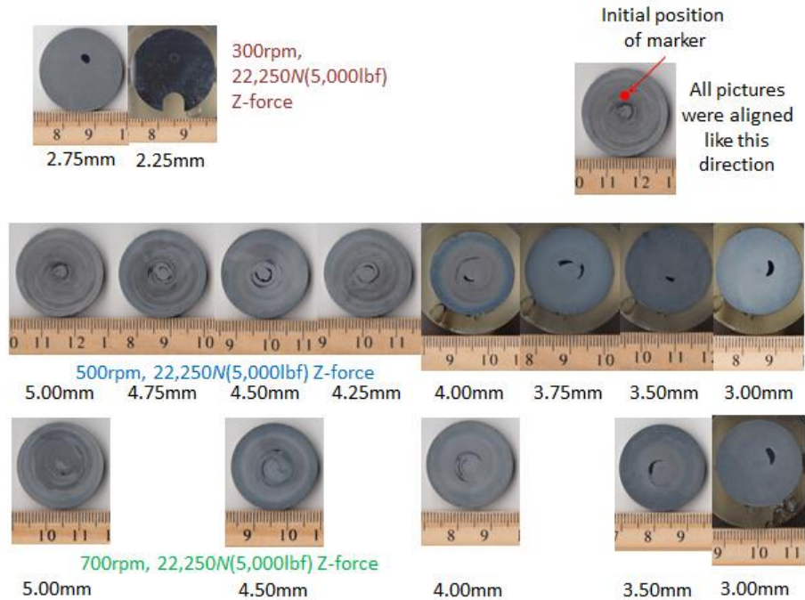
Figure 4.17 Material deformation of MA956 with stainless steel marker on 1/3r in Friction Stir Process, labeled with layer distance to the bottom of processed disc.
