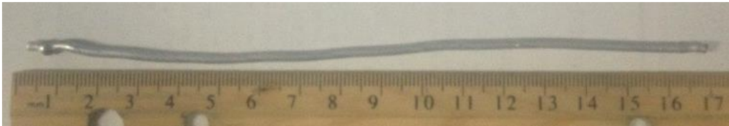
Figure 3.16 AA6061 wire made with friction extrusion, 300 RPM die rotational speed, 44500N extrusion force.
