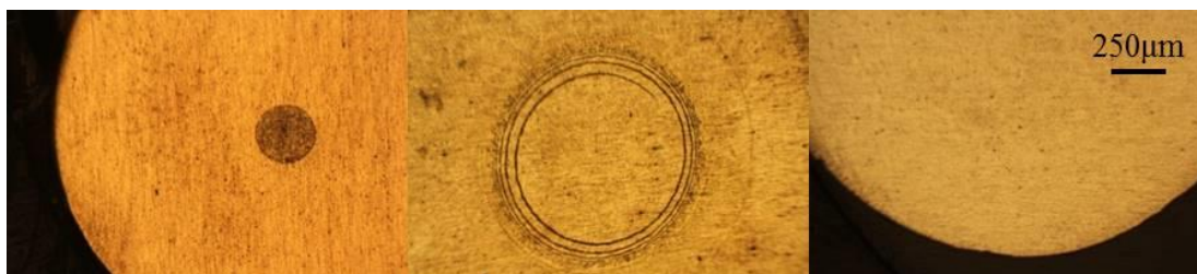
Figure 3.20 Bottom cross-section of scroll die extruded wire (left) Center marker, (middle) 1/3 radius marker, (right) 2/3 radius marker
