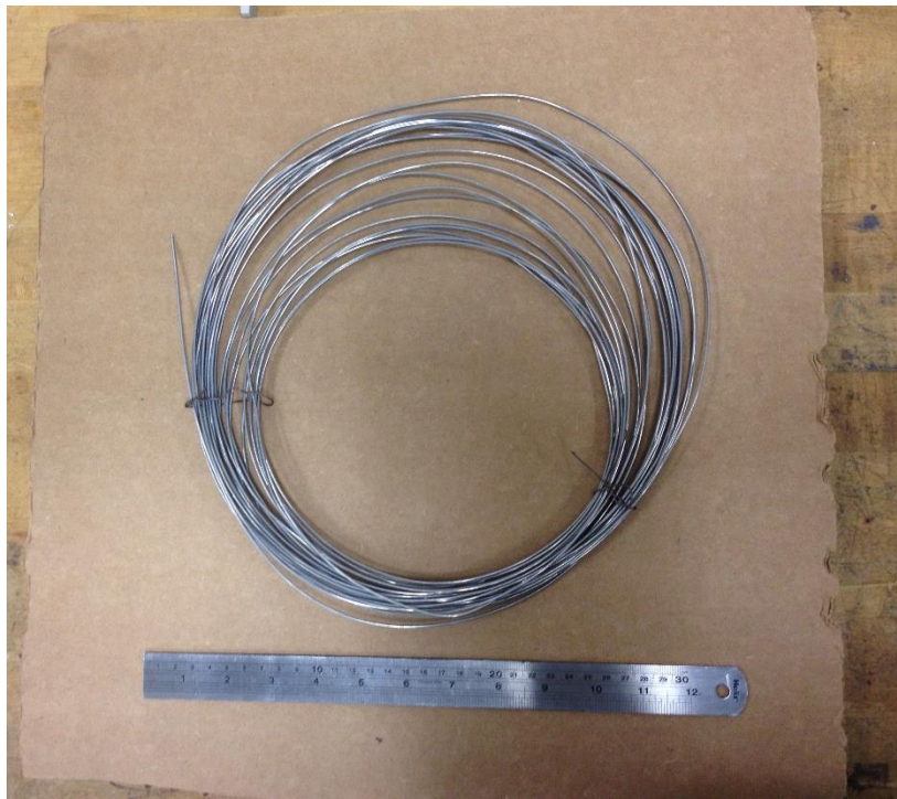
Figure 3.60 AA2050 drawn friction extrusion wire, 1.6mm in diameter
