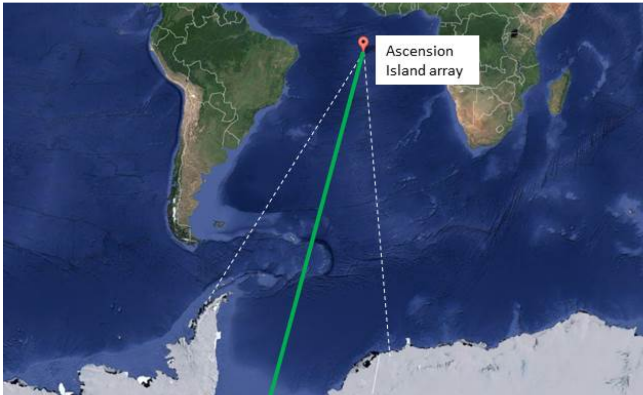
Figure 37: The projection of the main lobe of the plane wave beamformer upon the map. The green line is the center of the main lobe, and the dashed lines show the width of the lobe.
