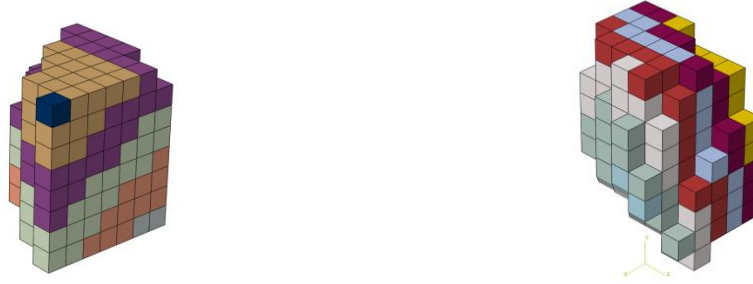
Figure 99. A comparison of a grain with a band width of two elements in thickness (left) compared to a grain of similar size but with a band width equal to a single element in thickness (right). Each band of elements is represented by a separate color.
