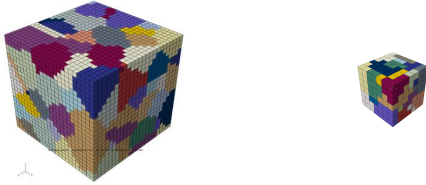
Figure 101. A comparison of the refined (left) and coarse (right) meshes used to assess the mesh dependence of the Stage II algorithm.
