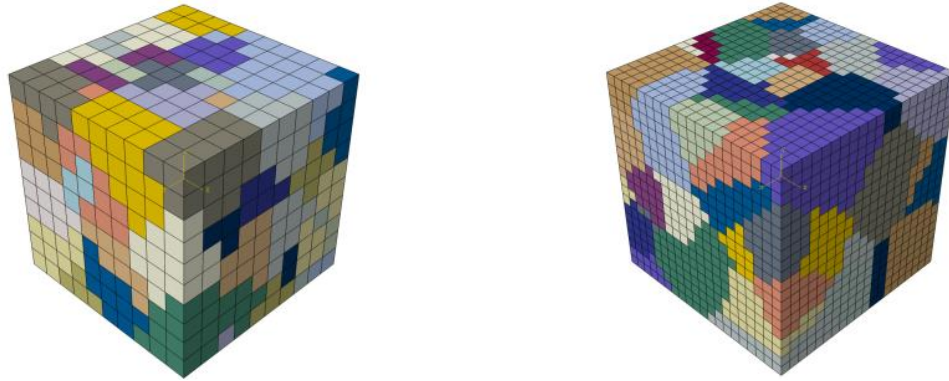
Figure 93. Coarse mesh with 5 \mu\text{m} elements (left) compared to a refined mesh with 2.5 \mu\text{m} elements. Both mesh configurations have the same volume and number of grains.
