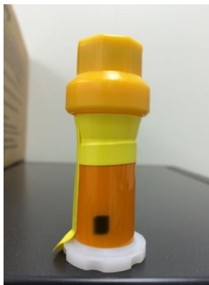
Figure 5.5. Sample container wrapped in photo paper to determine the active area of the irradiating x-rays from the x-ray tube.
