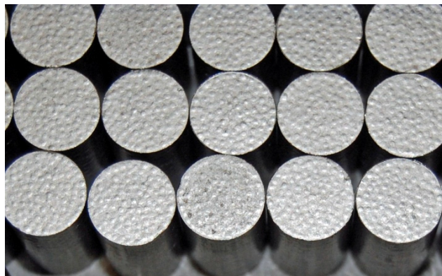
Figure 2.4: A completed cylindrical compact. Can see TRISO particles on surface [12]
