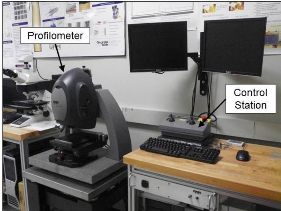
Figure 2.15 - The Zygo NewView 6k scanning white light interferometer (non-contact optical profilometer) used to measure the aluminum deposition.
