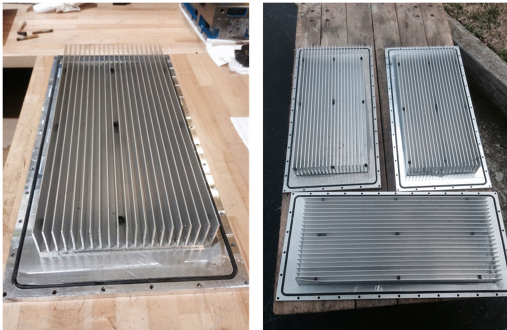
Figure 43. Assembled mounting plates for 1 MVA thermosiphon
