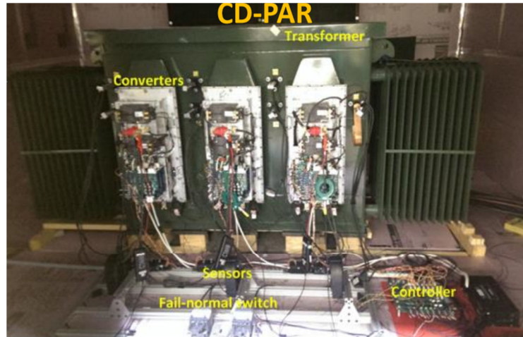
Figure 47: GCD-PAR thermosiphon-transformer assembly in the thermal chamber prior to testing
