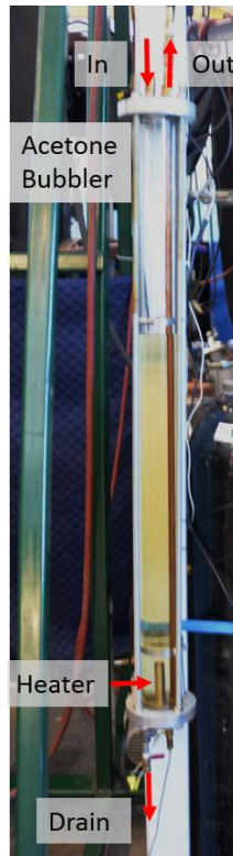
Figure 16: Acetone bubbler equipped with heater for seeding light gas with acetone.
