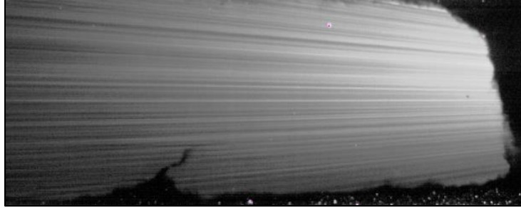
Figure 50: N_2/SF_6 , M=1.55 , \theta=60^\circ , PLIF image after reshock ( t\sim 8 ms).
