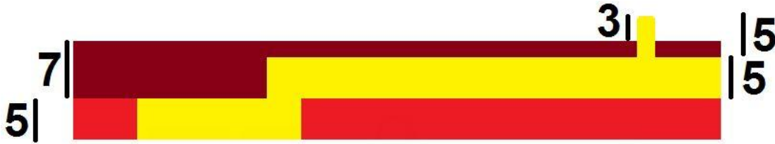
Figure 4.18 Cross-section schematic of the polyimide interconnect. The two red layers are polyimide and the yellow color represents gold metal layers.
