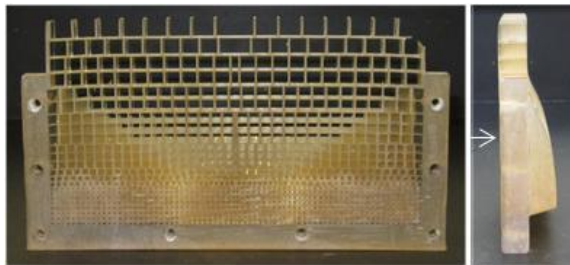
Figure 8.3 A honeycomb fence designed for thickening of the diffuser's inlet boundary layer.
