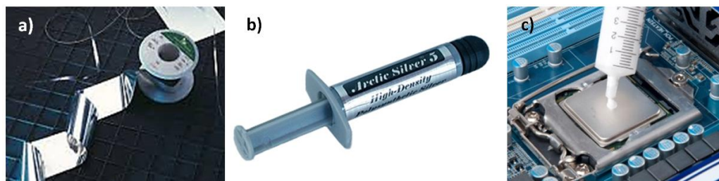
Figure 2.2: (a) roll of solder film [49] (b) thermal grease [50] (c) application of thermal grease to a heat spreader [51].
