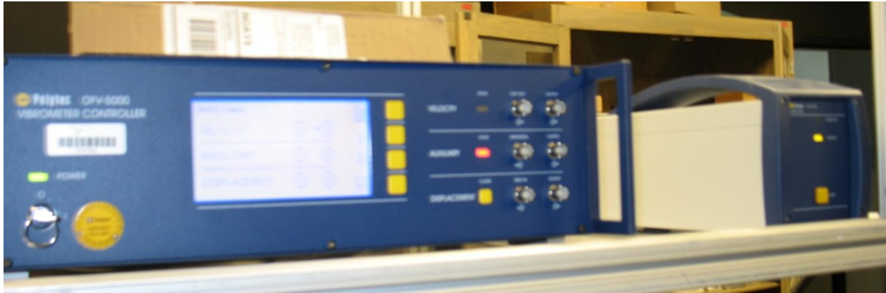
Figure E.10 Laser controller on left with the power key in the lower left. The right box is the laser power supply which is toggled by the yellow button.
