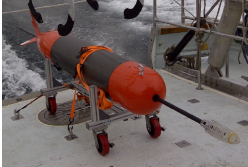
Figure 1: An autonomous littoral glider by Alaska Native Technologies (ANT-LLC), fitted with a vector sensor mounted inside a cage approximately one meter off the nose.
